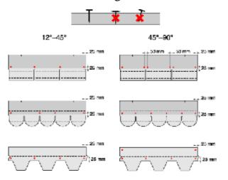
The nails are put 2-3 cm from the edge of the tile. Picture on the left indicate the number of nails needed and where they should be applied at certain roof angle. The picture shows the topside of the tile, and the dotted line indicates the place of the adhesive bottom layer.
