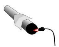
ATTENTION: if ridge – cornice tiles are installed at the outside temperature — lower than 10°C it is recommended to bend them on a heated 10 cm diameter tube in order to avoid cracks. (See the picture on the left)
