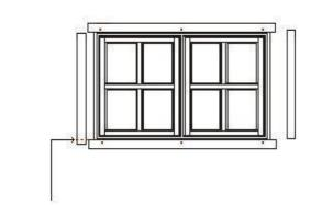
cut side pieces to fit as necessary, then screw to frame as before
