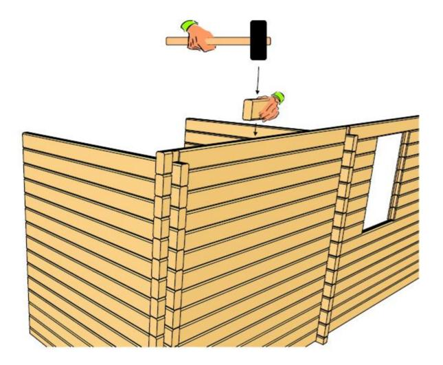
It is advisable to use a spirit level during the construction of the cabin. Using the Installation guide together with the Parts List for reference you can start erecting the walls. Beginning with part No. 1-1-BA and 1-2-BA for the back and front walls and following the installation Guide, fit the boards' one on top of the other. Ensuring the corners lock. Again it is advisable to use a spirit level during this process.
