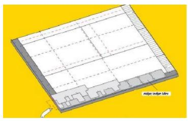
Ridge/cornice tiles or the usual tiles (with the jagged edge cut off) are used for the initial row of tiles along both the eaves of the roof as well as the pitched cornice at the top.
