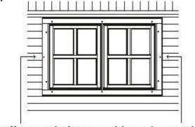
offer up window to cabin and screw in either side to cabin wall to hold in place
