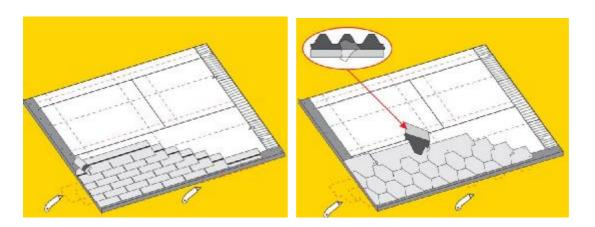
Ridge/cornice tiles should be cut into three parts at the places of perforation and laid in a straight line with an overlap of 3-5 cm. They are fixed with two nails on each side of the slope.
